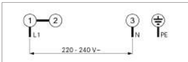
Fig. 4.87 1-phase connection diagram
